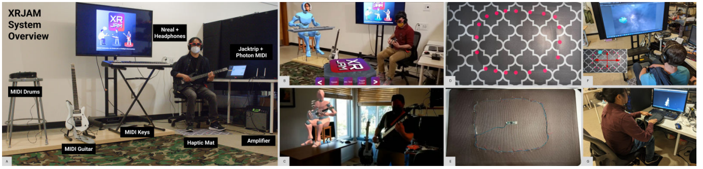
Fig. 1. A) XR Jam system overview and components. B) XR Jam through AR glasses. C) Guitar player jamming with guitar playing AIVM. D) View of the haptic mat top down. E) View of haptic mat motor arrangement. F) Spatial sound location pilot setup. G) Just noticeable difference pilot with avatar onscreen.
